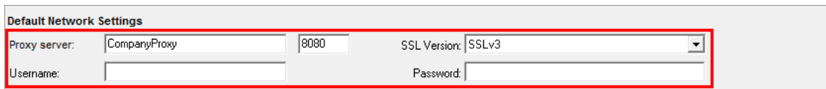
Figure 66: Settings for connecting to the internet over a proxy server in Server Manager
